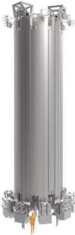
Fully assembled, the Central Solenoid, the largest of ITER’s magnets, will be 18 meters (59 feet) tall and 4.25 meters (14 feet) wide, and will weigh a thousand tons.
