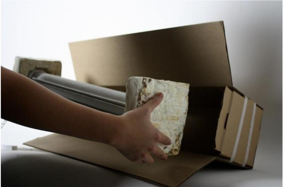
The new composite, called *EcoCradle*, is sustainable, structurally strong, and fire-resistant, requires almost no energy to produce, leaves no waste, and is biodegradable.
